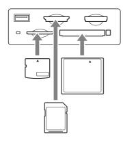
With the label facing up, fully insert the card in the direction indicated by  $\triangle$ .
